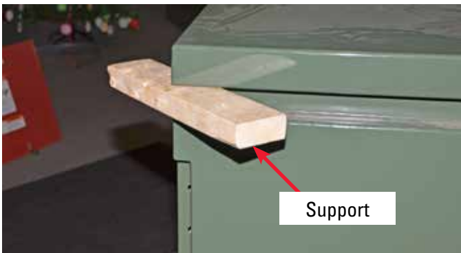
Figure 5. Wood block support installed at corner, initial location.
