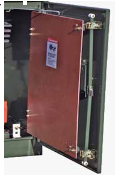
Figure 12. Three-point door latch mechanism. Enclosure door is secured open by windbrace. Inner barrier is secured open by a pin on the door inserted into a clip on the barrier.
