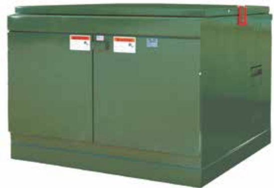
The Type PLD Pad-mounted Switchgear includes load-interrupter switches with terminal pads accommodating conventional terminators for a live-front interface and 200 ampere fusing with bushing wells accommodating 200 ampere load-break elbows for a dead-front interface. All units use the same fully tested and field proven switch designs.
