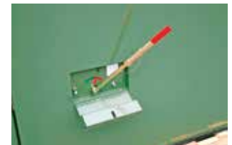
Figure 14. Remove handle. (Handle is attached by a cable.) Unfold handle and slide clip over pivot joint to secure handle in the extended position.
