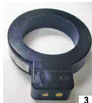
Figure 17a. The self-powered relay components include (1) the relay that provides all the settings and controls necessary to initiate vacuum fault interrupter operations based on the programmed parameters, (2) the magnetic actuator pictured that provides mechanical trip-actuation of (and is mounted on) the vacuum fault interrupter mechanism and (3) the current-sensing transformer that provides sensing and power input to the relay and trip circuit.
