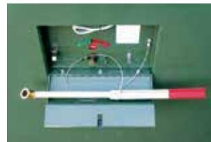
Figure 9. Remove and unfold handle. Secure handle in the extended position by sliding clip over joint of handle sections.
