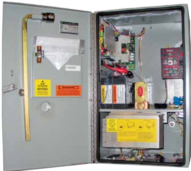
Figure 20. Fast-Trip Style motor operator has a large, high-speed motor and space to accommodate an array of communications and control components similar to that of the Run-and-Trip motor operator. The cover over the motor is interlocked so that when the cover is opened, the motor will not operate to avoid exposure to fast moving parts. Other features are similar to those shown for the Run-and-Trip motor operator.
