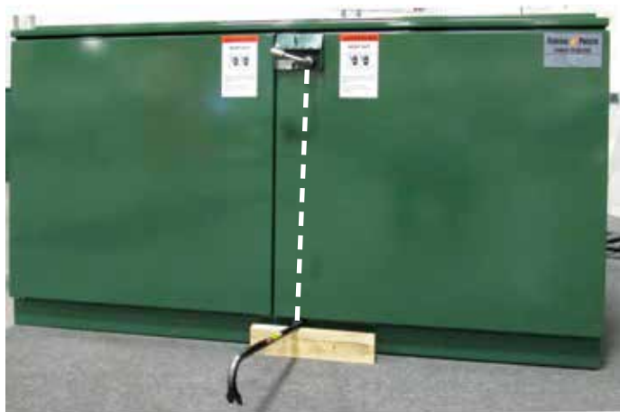
Figure 5. Gently pry up active door at bottom in line with the latch assembly. The penta-bolt can be used to approximate the correct location.
