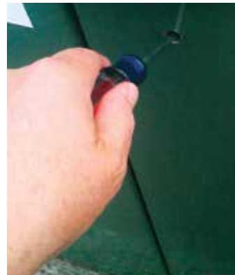
Figure 3a. With the flat edge of the screwdriver horizontal, insert the screwdriver through hole drilled in door.
