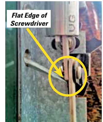
Figure 3b. Flat edge of screwdriver positioned under latch-bar joint.
