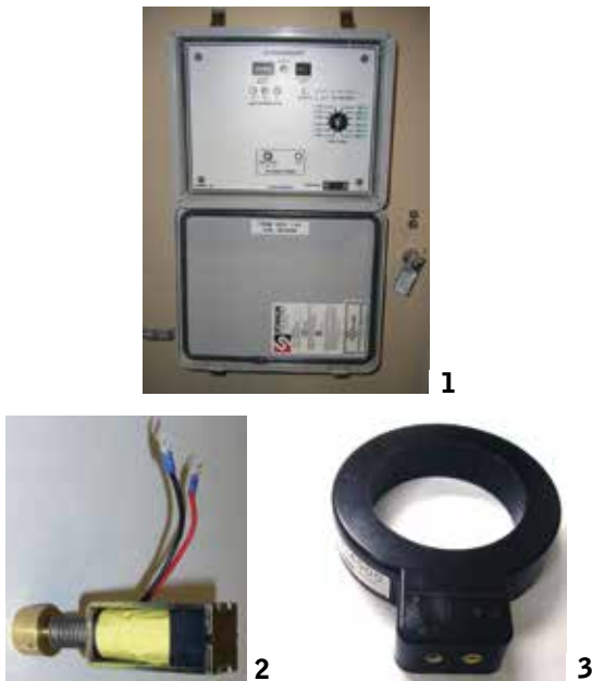
Figure 10. The self-powered relay components include (1) the relay that provides all the settings and controls necessary to initiate vacuum circuit-breaker operations based on the programmed parameters, (2) the magnetic actuator pictured that provides mechanical trip-actuation of the vacuum circuit-breaker mechanism and (3) the current-sensing transformer that provides sensing and power input to the relay and trip circuit.
