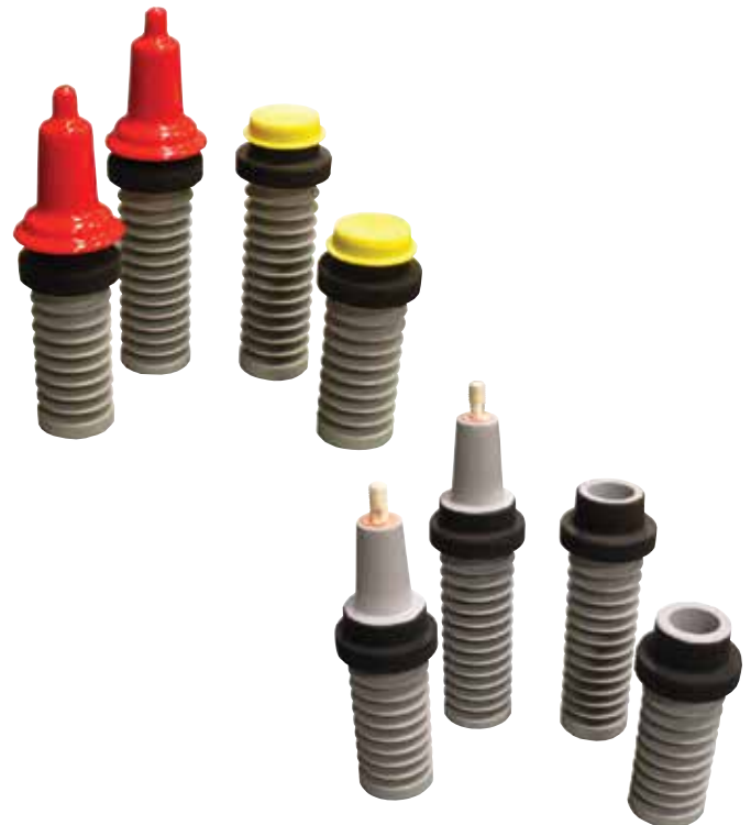
Figure 9. Federal Pacific cycloaliphatic bushings and bushing wells have all copper conductors and silver-plated removable studs. Semi-conductive coating isolate bushings and dust covers protect high-voltage interfaces.
