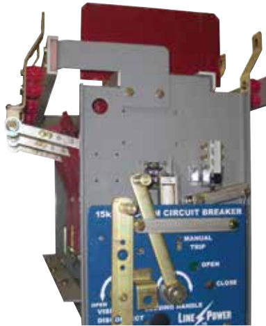
Figure 2. Federal Pacific's 15kV, 600 ampere magnetically-actuated vacuum fault interrupter switch for use with a self-powered relay includes an integral visible disconnect . Disconnect shown closed.
