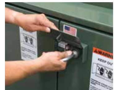
Penta-head (or optional hex-head) actuated door lockbox features stainless-steel hinged padlockable cover to block access to bolt head. Rotate bolt in either direction for opening.
