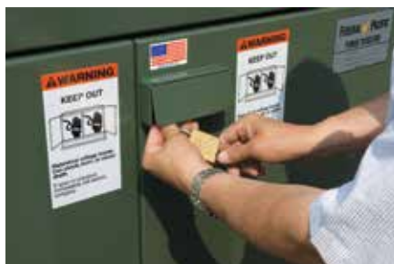
Penta-head (or optional hex-head) actuated door lockbox features stainless-steel hinged padlockable cover to block access to bolt head. Rotate bolt in either direction for opening.
