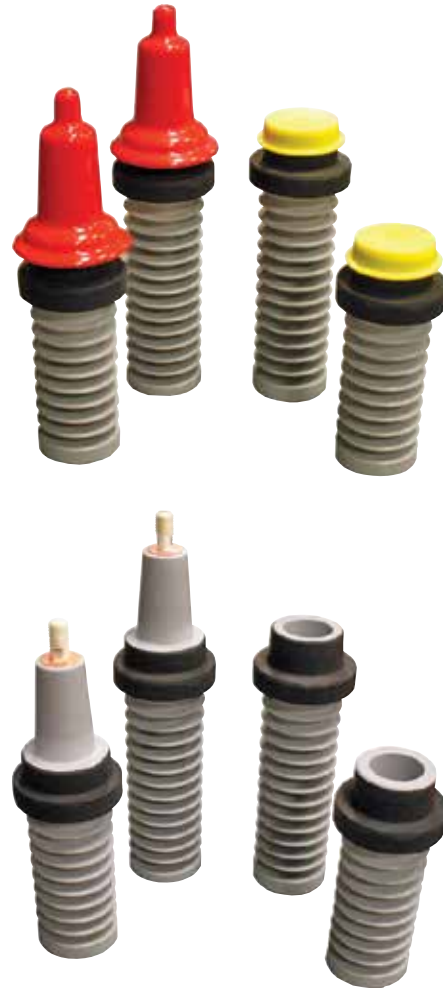
Figure 9. Federal Pacific cycloaliphatic bushings and bushing wells have all copper conductors and silver-plated removable studs. Semi-conductive coating isolate bushings and dust covers protect high-voltage interfaces.
