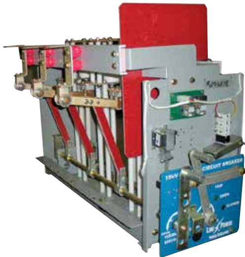
Figure 3. Federal Pacific's 15kV, 600-Ampere Vacuum Fault Interrupter With Visible Disconnect For Use With Overcurrent Relays That Require External Control Power. Disconnect Shown Closed.
