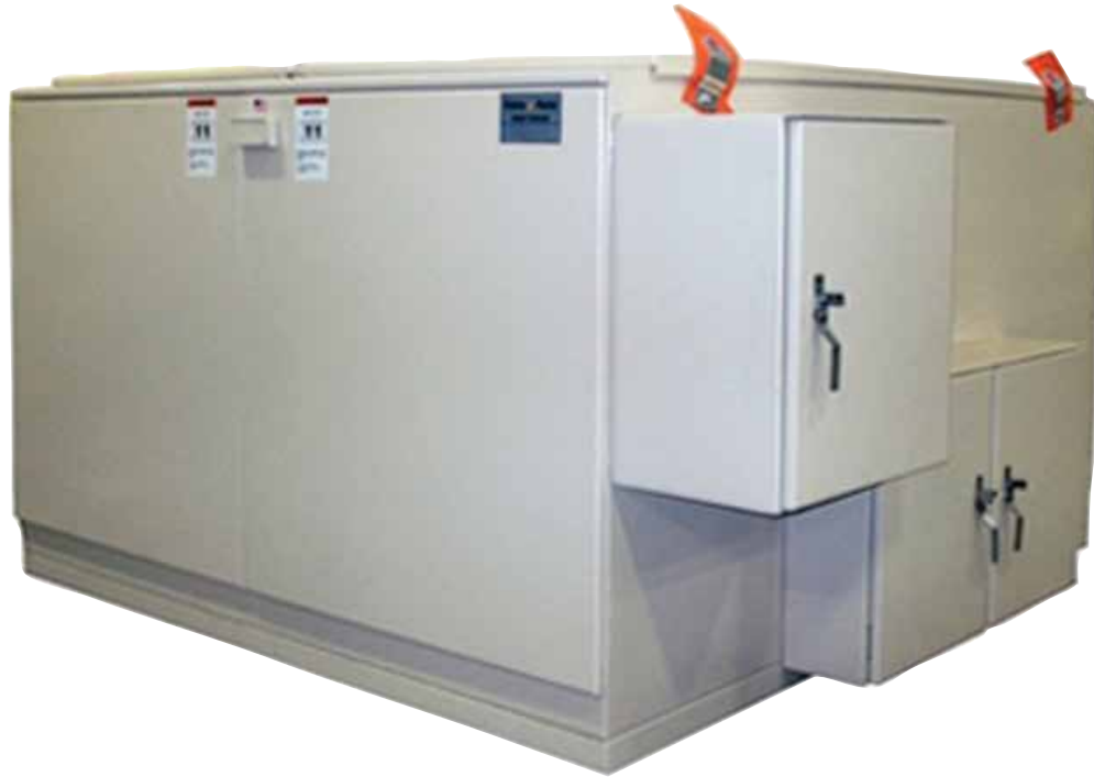
Figure 1. Federal Pacific PVE Models Incorporate Vacuum Interrupters With Visible Disconnects Into A Rugged Heavy-Gauge Steel Enclosure Featuring Air-Insulated, Dead-Front Construction.
