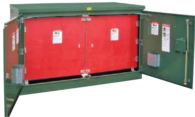
Figure 3. Open door view of the FUSE compartment showing the internal, hinged and bolted barriers of NEMA grade GPO-3 red fiberglass barriers that provide isolation from energized components. Clear polycarbonate barriers are available as an option.
