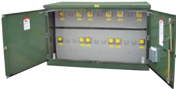
Figure 2. The ELBOW compartment includes bushing wells for connection of (the normally customer furnished) inserts and elbows. At the top are the bushing wells for the incoming (source) circuit connections with an IN and OUT position for each phase and a parking stand between them. At the bottom are the bushing wells for the outgoing (load) circuit connections (two fuses per phase) and a parking stand is provided for each outgoing circuit.
