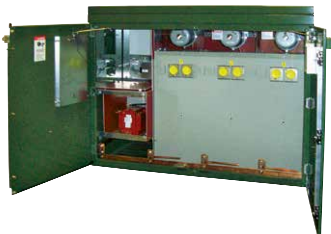
Figure 2. Dead-front compartment with bushing wells to accommodate inserts and elbow connectors (not furnished) for cable entry. Units are furnished with clear polycarbonate barrier in dead-front compartment to permit viewing vacuum interrupter targets.
