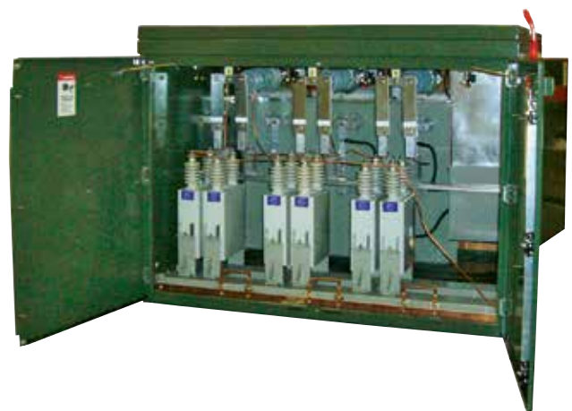
Figure 3. Live-front compartment of pad-mounted capacitor bank. Unit is shown with front barrier over fused voltage transformer and compartment front barriers removed. Red GPO-3 fiberglass barriers are standard. Optional clear polycarbonate barrier in live-front compartment, which provides enhanced visibility over standard red fiberglass barrier, are available.
