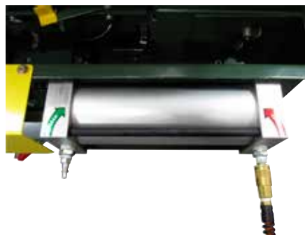
Figure 7. Top view of PROM-PM with hose connected to port on right.
