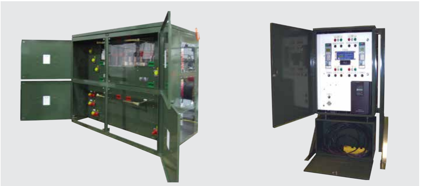
Figure 5. A Custom Solution configuration of four MAVRiC® units is arranged in a vertical orientation (at left) to match available space in an existing above-grade uncovered vault and to replace SF6 gas-insulated equipment that was prone to leaking and vulnerable to the environment. The relay and control package (at right) is designed to be wall-mounted independent of the switchgear and is also provided with a symbiotic hand-held controller to allow local operations to be performed outside the vault and outside the arc-flash boundary, allowing for maximum security for operating personnel.
