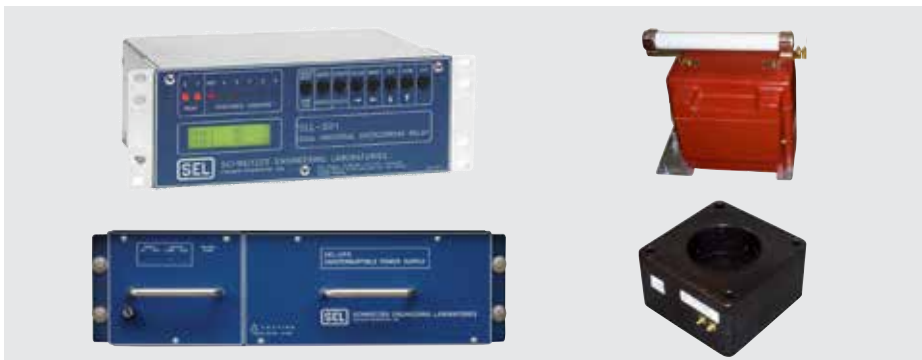
Figure 8. The overcurrent protection scheme implemented with the SEL relay includes (1) the SEL-501 Dual Universal OCR, which handles two load feeders; (2) a fused voltage transformer to provide control power for the relay and MAVRiC® units; (3) a UPS for backup power if control power is lost and (4) current transformers to sense the overcurrent condition and provide that input to the SEL relay for interpretation and action.
