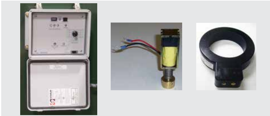
Figure 7. The self-powered relay components include (1) the relay that provides all the settings and controls necessary to initiate vacuum fault interrupter operations based on the programmed parameters; (2) the magnetic latch that provides mechanical trip actuation of (and is physically mounted on the frame of) the vacuum fault interrupter; and (3) the current transformers that provide sensing and power input to the relay and trip circuits and that are mounted on the power cables.
