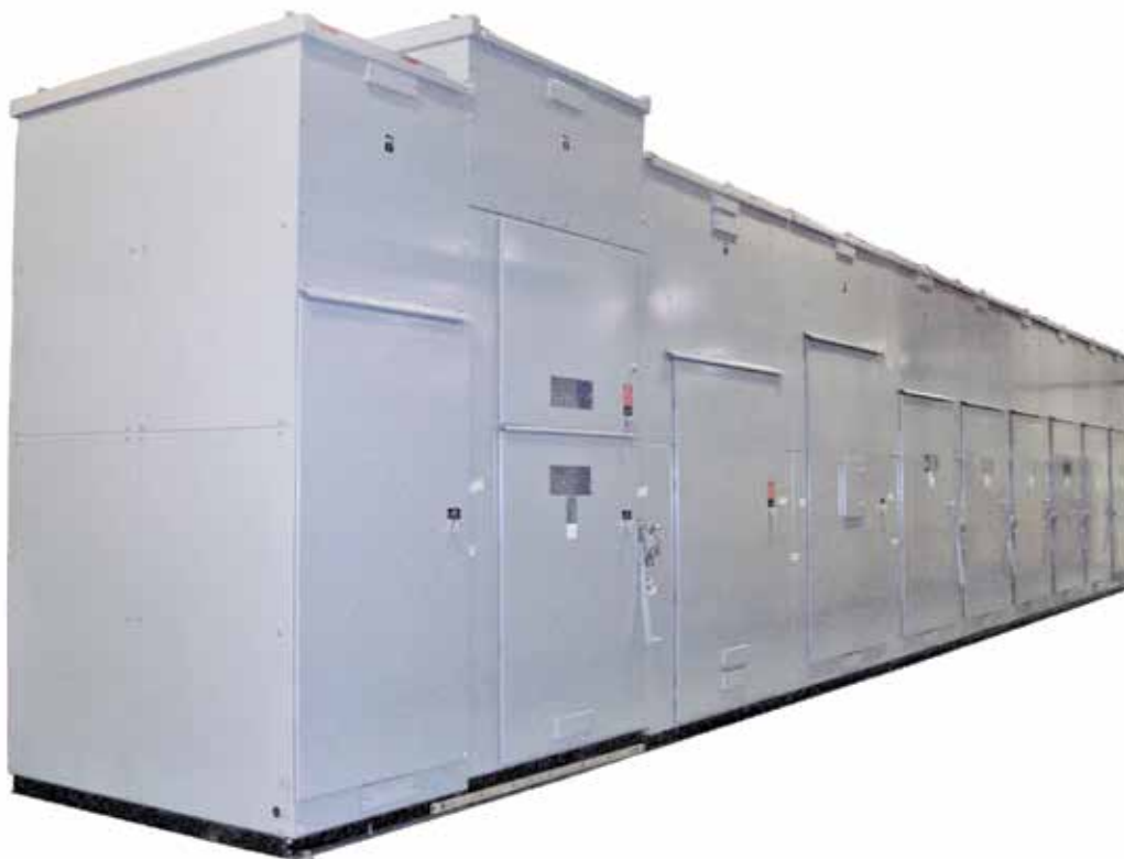
Figure 1. This 10-bay lineup of 38kV Metal-Enclosed Switchgear provides switching and protection at a major installation in the Northeast. The switchgear assembly includes: a billing metering compartment, a cable-entrance compartment, a main-circuit breaker compartment with Auto-jet® Switch as a visible disconnect, utility metering bay, customer metering bay and six (6) fused-switch feeder bays.
