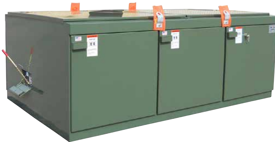
Figure 1. Air-insulated 15.5kV 6-compartment dead-front pad-mounted switchgear unit provides a compact, multi-functional, front-end metering installation for this overhead to underground conversion project, replacing an obsolete and unsightly overhead metering installation. The coating system on the switchgear unit provides long-term environmental protection, while the dark-green color allows the pad-mounted switchgear to blend unobtrusively into the state park setting. This type of pad-mounted metering is ideal for any application where primary metering of bulk power is required, such as at factories, commercial centers, business parks, and, in this application, recreational areas.
