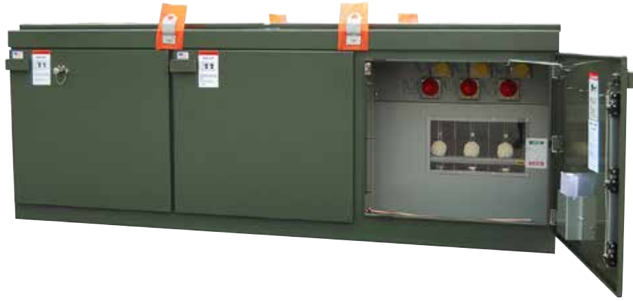
Figure 3. Incoming switch termination compartment, featuring a wide mar-resistant polycarbonate viewing window, allows direct view of switch blade position. Clearly visible open/closed labels and supplemental switch position indicator help to orient and identify blade position. In addition to the standard 600-ampere bushings, customer requested optional 200-ampere bushing wells (one in parallel with each bushing) to provide convenient locations for grounding or installing surge arresters.
