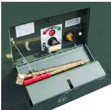
Figure 4. View of the stainless-steel switch-operating handle pocket. The bracket shown over the hex switch-operating shaft is an example of the “-K2” option, which allows the switch to be locked into the open or closed position when the bracket is padlocked across the switch-operating shaft. To the right of the switch-operating shaft is an example of the “-K3” key interlock option, which prevents opening of the fuse termination compartment doors unless the loadbreak switch is in the open position.
