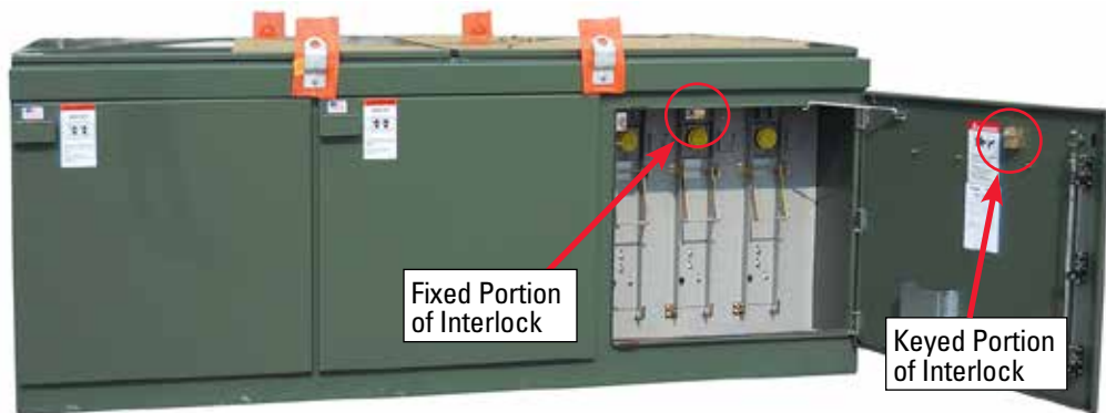
Figure 8. View of load fuse-termination compartment. Fuse panels hinge at bottom, providing full isolation at both sides of the fuse assembly when in open position, while allowing ground and drain wires to be maintained, and insulating protective caps remain installed, during the fuse panel operation sequence. Dual viewing window in each hinged fuse panel allow viewing of the blown-fuse indicator target and fuse size information. The keyed portion of the fuse-termination compartment interlock is on the door, while the fixed portion of the interlock is at the top of the compartment door opening, as shown.
