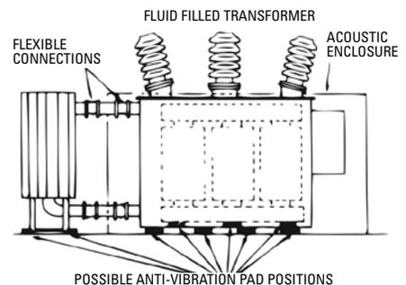
TYPICAL TRANSFORMER CONNECTIONS
