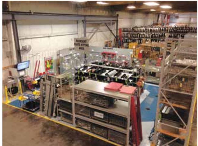
**Figure 14 After** – Kitting area, using Kanban stocking system.
