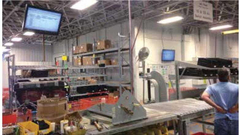
**Figure 10** – Monitors in the switch assembly shop show the enclosures being completed. This provides the "schedule" for producing switch and fuse component assemblies that are to be installed in those specific enclosures.
