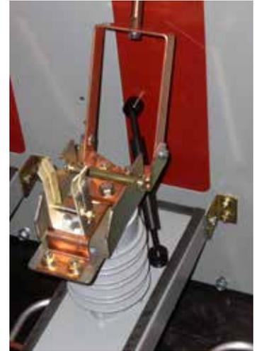
*Figure 10. Federal Pacific has developed a new turnbuckle, which is connected between the fuse panel and the red GPO-3 fiberglass shutter barrier. The enhanced design (in black) has increased mechanical capability and is easier to install, remove and replace. It can be used to replace installed earlier-design turnbuckles, requiring only the addition of a suitably-sized hole in the barrier.*
