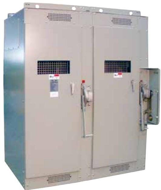
*Figure 20. Metal-enclosed switchgear (and pad-mounted Switchgear not pictured) is shown equipped with a Federal Pacific Portable Remote Operating Mechanism on the bay at right to allow operation from a distance of up to 50 feet using compressed air or CO<sub>2</sub>.*
