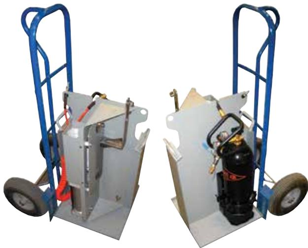
*Figure 19. Portable remote operating mechanism available from Federal Pacific can be mounted over switch-operating handle on switchgear stile and operated from a distance of up to 50 feet to open and close the switch using compressed air or CO<sub>2</sub>. Similar arrangements are available for pad-mounted switchgear.*
