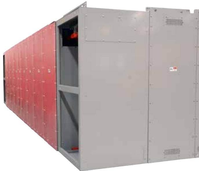
*Figure 18. Extending across the entire rear of the switchgear assembly are full-height sheets of GPO-3 grade red fiberglass. These insulating sheets, installed with non-metallic hardware, provide isolation of the metal switchgear surfaces from adjacent energized components that are located in the vault where the equipment will be installed.*
