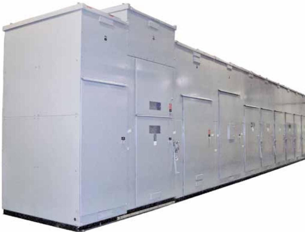
*Figure 1. This 10-bay lineup of 38kV Metal-Enclosed Switchgear provides switching and protection at a major installation in the Northeast. The switchgear assembly includes: a billing metering compartment, a cable-entrance compartment, a main-circuit breaker compartment with Auto-jet<sup>®</sup> Switch as a visible disconnect, utility metering bay, customer metering bay and six (6) fused-switch feeder bays.*
