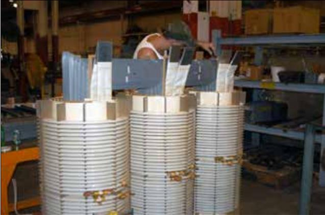
Figure 16. Insertion of top yoke.
