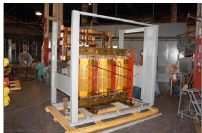
Figure 20. First stage of final assembly.
