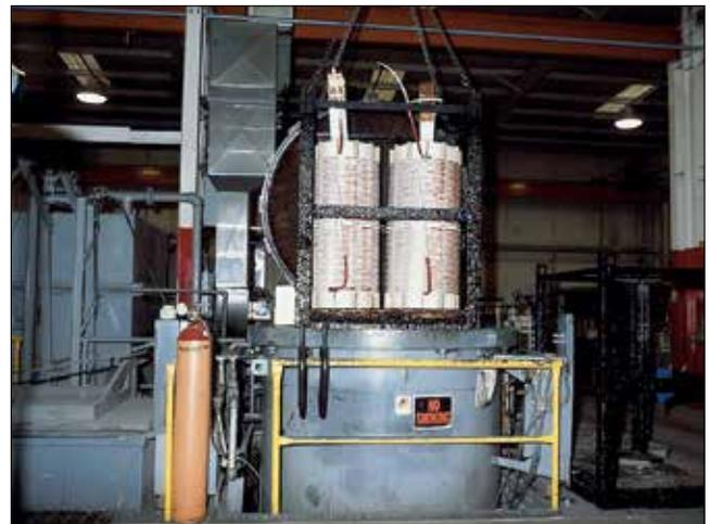
Figure 9. Coils after VPI process ready for baking in the oven.
