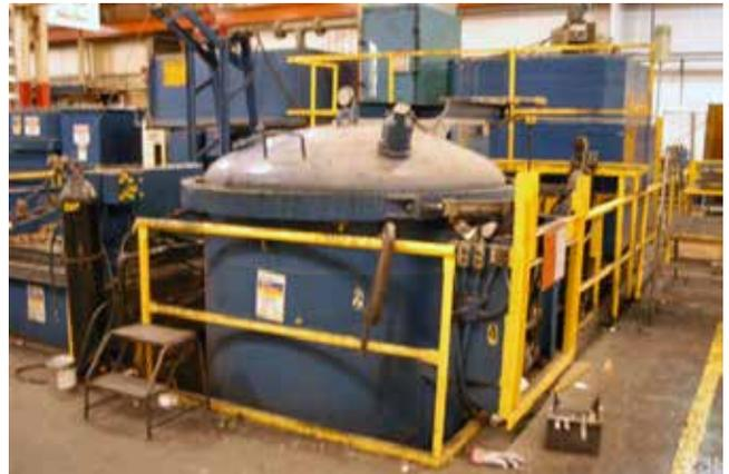
Figure 8. Pressure rated vessel for VPI
