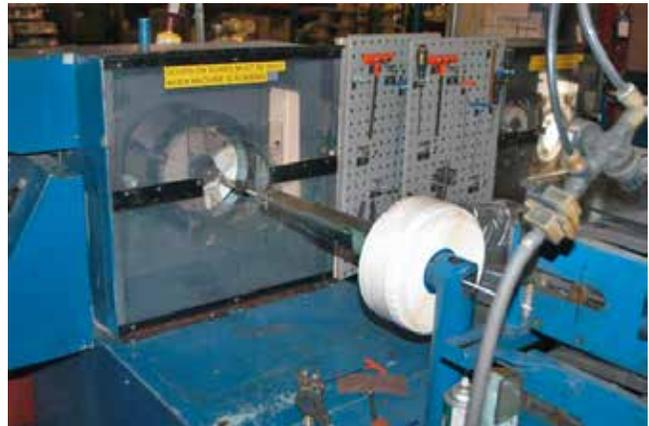
Figure 3. Nomex<sup>®</sup> tape being wrapped on the coil conductor.
