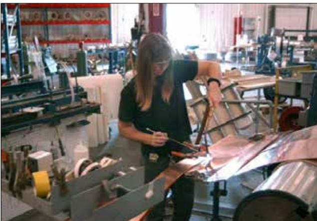
Figure 6. Copper brazing LV coil to LV lead.
