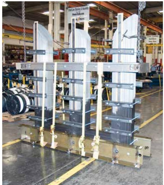
Figure 15. Step-lap mitre core ready for coils.
