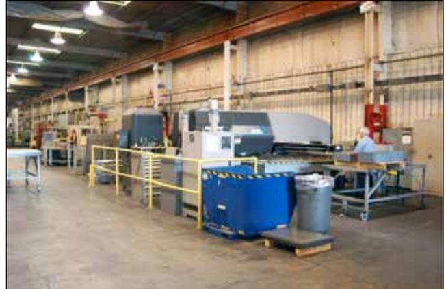
Figure 17. Metal fab facility (shearing, punching, and bending).
