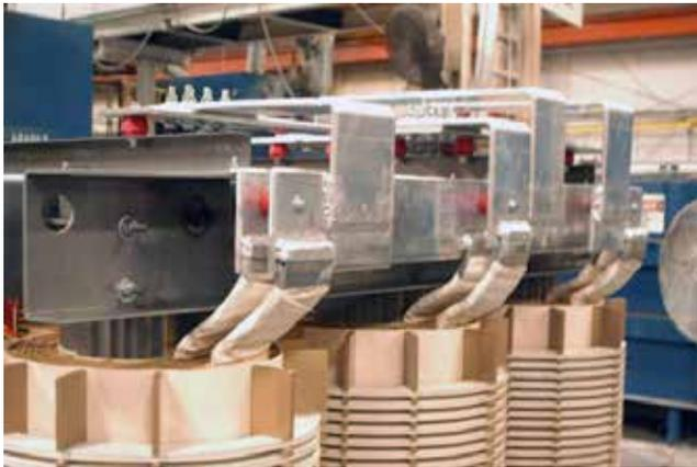
Figure 5. MIG welded leads to AL bus.
