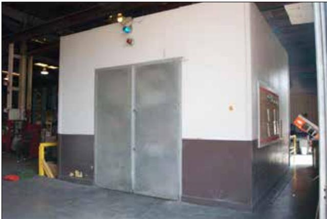
Figure 23. Large anechoic sound test chamber.
