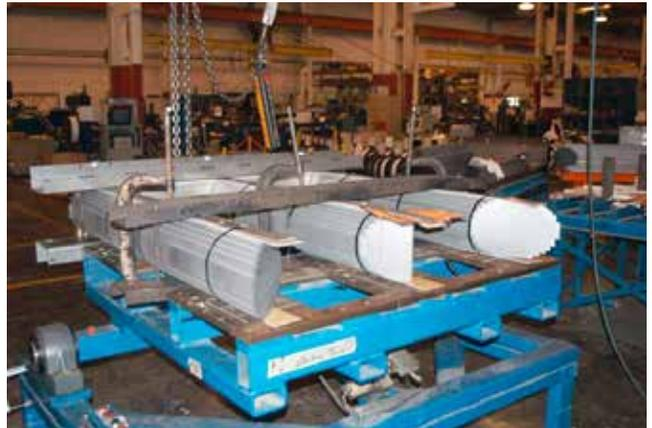
Figure 14. completely stacked core on rotatable table.
