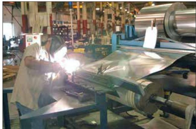
Figure 4. TIG welding LV coil to LV lead.
