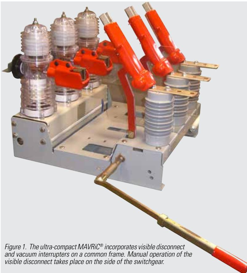
Figure 1. The ultra-compact MAVRiC® incorporates visible disconnect and vacuum interrupters on a common frame. Manual operation of the visible disconnect takes place on the side of the switchgear.
