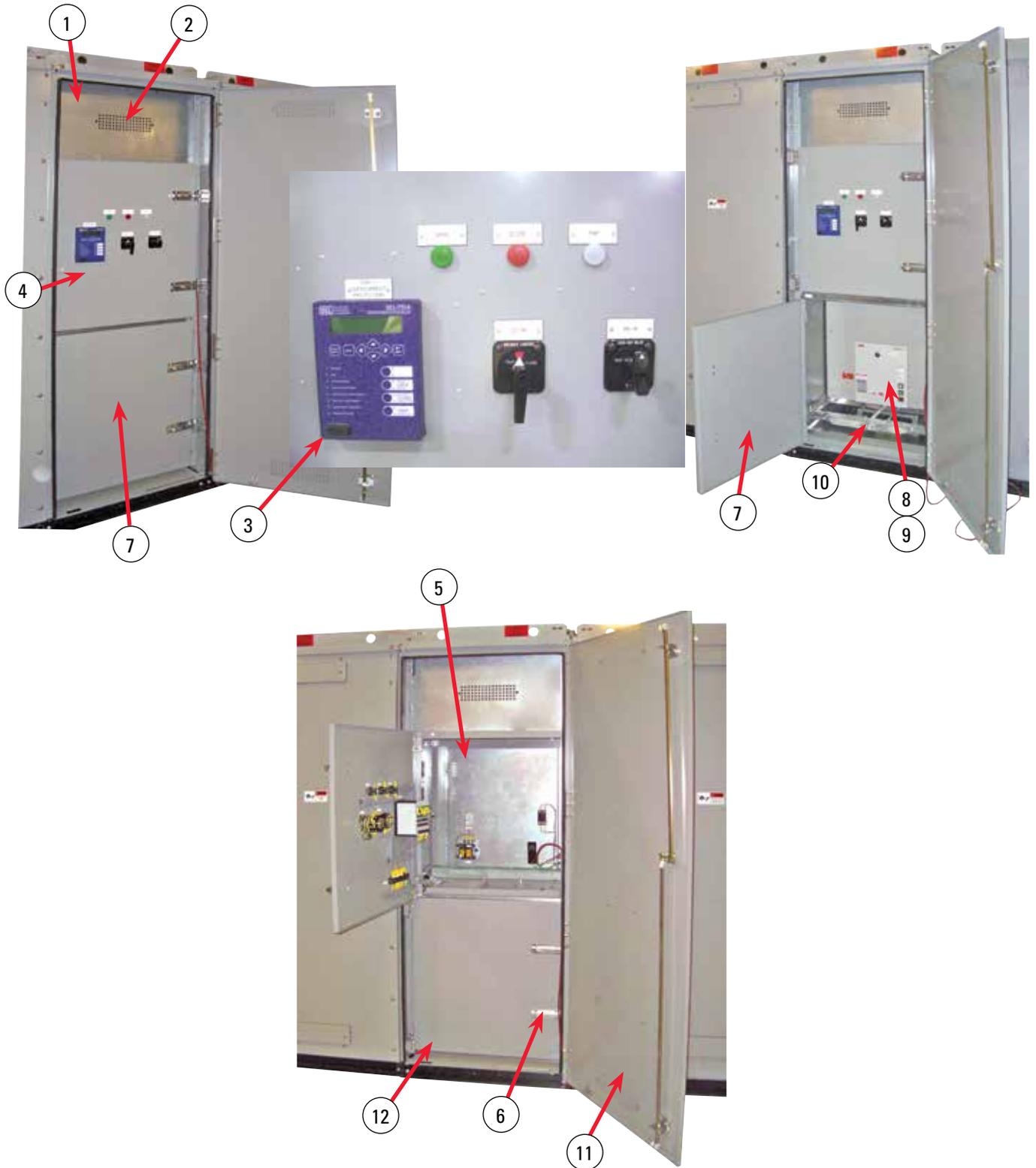
Figure 3. Bay 2 is the switching and protection compartment that includes the drawout VCB, the overcurrent relay, the sensing CTs that detect the overcurrent condition and all the associated low-voltage controls. The ground bus is continuous throughout all bays at both the front and the rear. In addition, an insulated terminal is provided in this bay (and in bays 1, 2R, 3 and 3R) for terminating concentric-neutral cables and ground leads from secondary wiring.
