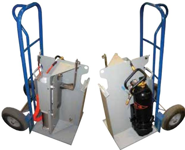
*Figure 13. Portable remote operating mechanism available from Federal Pacific can be mounted over handle on switchgear stile and operated from a distance of up to 50 feet to open and close the switch using compressed air or CO<sub>2</sub>. Similar arrangements are available for pad-mounted switchgear.*
