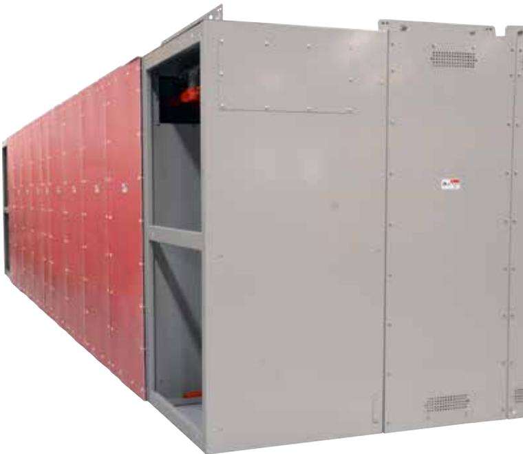
*Figure 12. Extending across the entire rear of the switchgear assembly are full-height sheets of GPO-3 grade red fiberglass. These insulating sheets, installed with non-metallic hardware, provide isolation of the metal switchgear surfaces from adjacent energized components that are located in the vault where the equipment is installed.*
