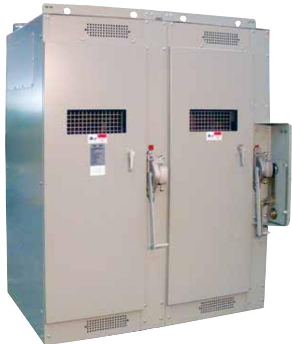
*Figure 14. Metal-enclosed switchgear (and pad-mounted Switchgear not pictured) is shown equipped with a Federal Pacific portable remote operating mechanism on the bay at right to allow operation from a distance of up to 50 feet using compressed air or CO<sub>2</sub>.*
