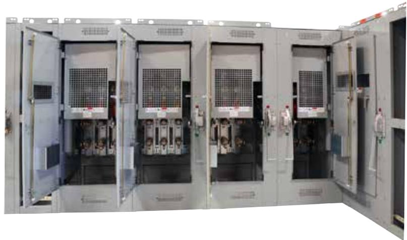
Figure 9. The photo at left shows an open door view of four (4) of the feeder bays on the right side of the bus-tie switch. Perforated steel screens over switches of feeder bays limit exposure to energized bus at the top of the bay when the switch is open and access to the interior is necessary, such as to change fuses.
