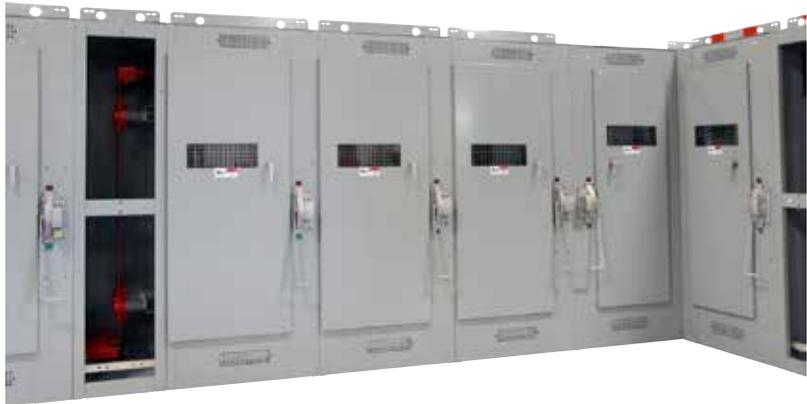
Figure 8. The five (5) feeder bays on the right side of the switchgear assembly are pictured at left. Doors of feeder bays include mechanical interlocks to prevent opening the door until the switch is open. With the doors open, access is possible to change fuses. While the door is open, the switch cannot be operated. Viewing window in each door allows inspection of the interior without requiring that the door be opened
