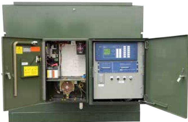
Figure 2 – In this view, the doors of the low-voltage cabinets are open, showing the standard run-and-trip motor operator in the cabinet to the left, and the control cabinet, featuring the SEL-451 relay, in the cabinet to the right. The control cabinet is shown in detail in Figure 6.
