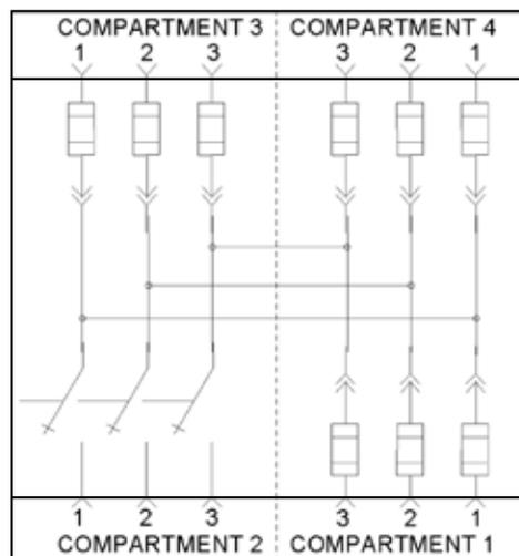
Figure 4. The above one-line diagram illustrates the 38kV PSE-12 configuration, which includes one 600-amp Auto-jet® Load-Interrupter Switch and three (3) three-phase sets of 38kV Federal Pacific fuse mountings, accommodating DBU fuse units, SMU-20 fuse units or CMU fuse units. And, the switchgear is furnished with Federal Pacific's FP-3097 end fittings which accommodate all of these fuse-unit brands.
