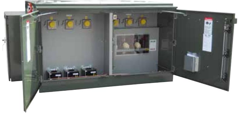
Figure 2. Open door view shows incoming termination compartment at right with incoming load-interrupter switch visible behind viewing window. Outgoing termination compartment is at left and includes sensing CTs to measure and confirm load current and provide that input to the power monitoring relay. The voltage transformers are mounted in the interior of the switchgear.
