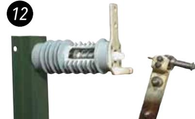
The arc is extinguished and there is a full dielectric air gap between the switch blade and the main contact.
