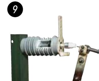
At the time of contact separation, not only is the discharging operating mechanism pushing the blade very fast, but the probe and puffer springs are applying energy to rapidly separate the interrupting contacts, which are only in the circuit for 1.5 cycles of the total operating time.
