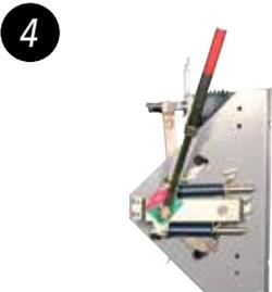
Switch opening. As switch blade continues to move, the probe and puffer springs are further compressed and the initial electrical change occurs as the switch blade starts to separate from the main-contact.
