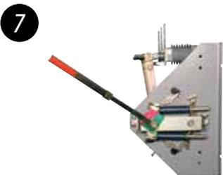
Interrupter contacts separate. As the springs are fully compressed, the probe and the tulip contacts will start to separate. The charged puffer spring now quickly pulls the puffer assembly, which includes the tulip contact, back into the pump-insulator chamber.
