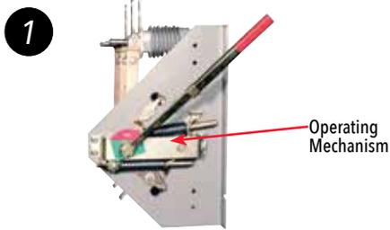
Switch closed. Normal current path through lower switch terminal, through switch blades to main-contact and out top terminal pad.
