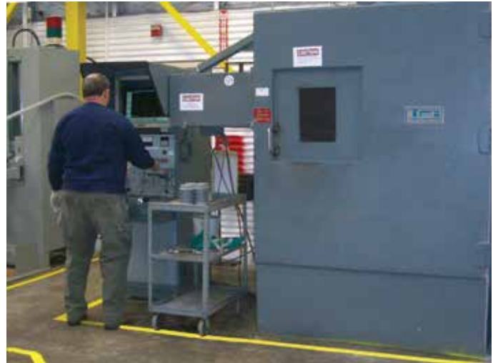
Finished insulators are 100%, 360°, end-to-end fully inspected internally by 100kV real-time fluoroscopic x-ray.
