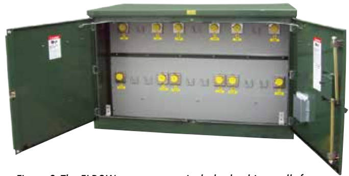
Figure 2. The ELBOW compartment includes bushing wells for connection of (the normally customer furnished) inserts and elbows. At the top are the bushing wells for the incoming (source) circuit connections with an IN and OUT position for each phase and a parking stand between them. At the bottom are the bushing wells for the outgoing (load) circuit connections (two fuses per phase) and a parking stand is provided for each outgoing circuit.
