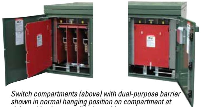
*Switch compartments (above) with dual-purpose barrier shown in normal hanging position on compartment at right and in alternate slide-in position on compartment at left. Barrier should **not** be left in alternate position for more than one week. Hinged B4 barrier shown on switch compartment at left.*
