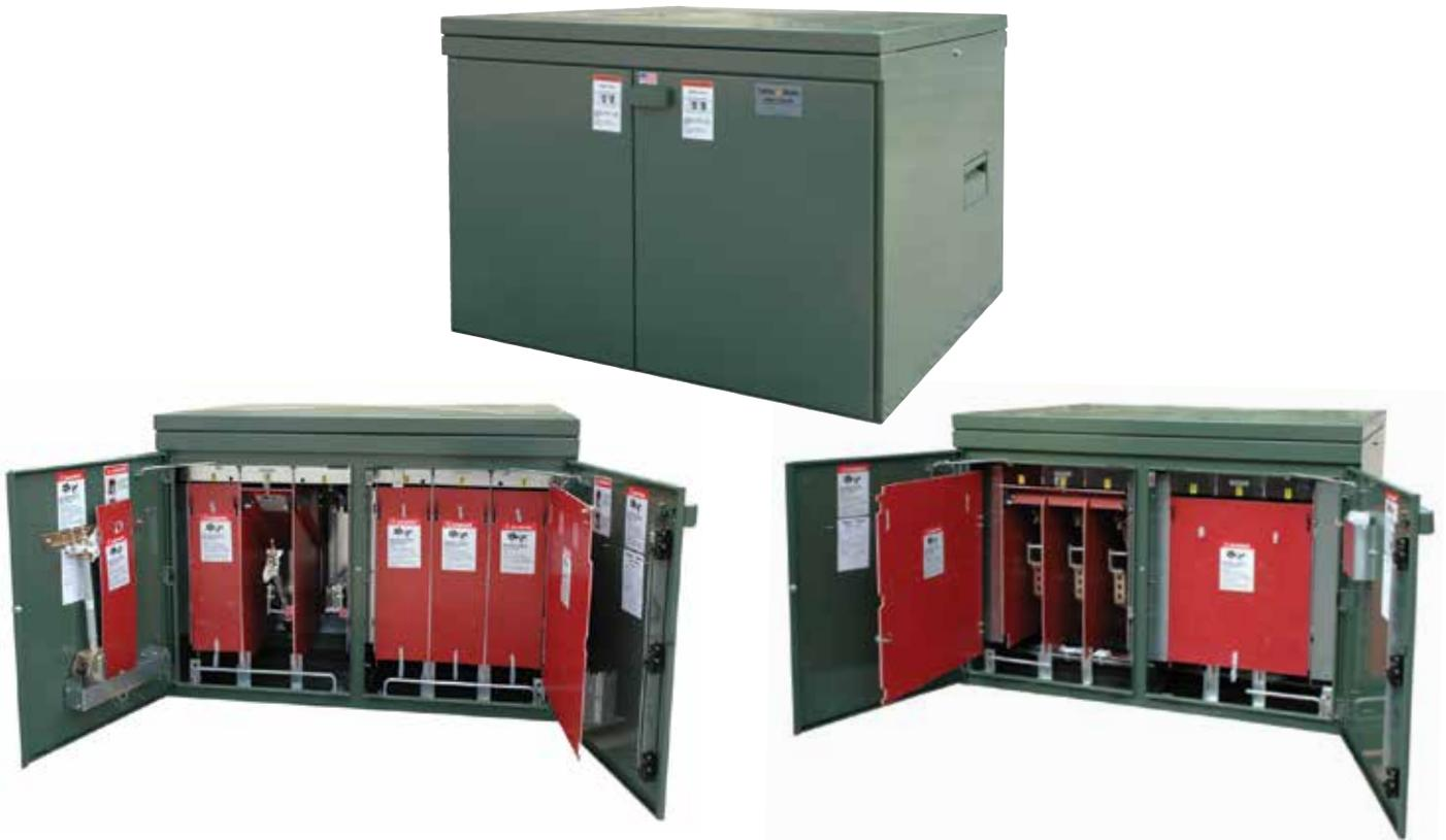
*The PSI/II Pad-Mounted Switchgear is Federal Pacific's line of live-front pad-mounted switchgear (available as UL® Listed) built to IEEE C37.74 requirements and features the fully tested and field proven Auto-jet® load-interrupter switch for switching three-phase circuits and the integral load-interrupter for single-phase load-break operation with fuses.*
