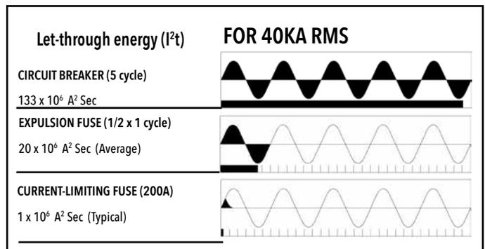
*Figure 1. The dark area under each curve represents the relative energy limitation of damaging let-through currents provided by various protective devices. The curves illustrate that fuses allow through much less damaging let-through currents and, therefore, do a much better job of protecting cables and transformers.*
