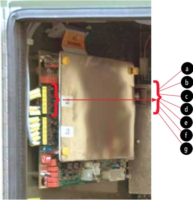
Figure 5. Control module with LED status lamps.
