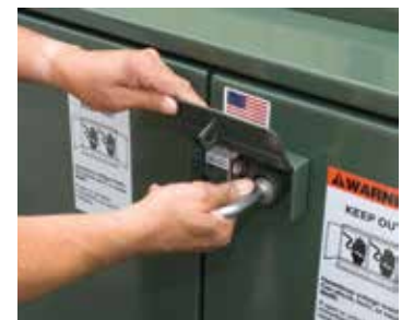
Switch-Handle Operation - handle unfolds and clip slides over joint to fix handle in extended position
